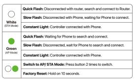
STA Mode - Controller connect to Home Router (Support Multiple devices connect and control)
